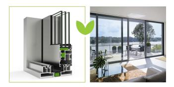
The added benefits are security and weather performance. When the door is in its locked position it has a multi-point lock securing your property but this is enhanced by "gravity" the full weight of the door and glass are resting on the track. Also, a fully closed door rests over lower weather seals improving the doors weather tightness and acoustic insulation.
